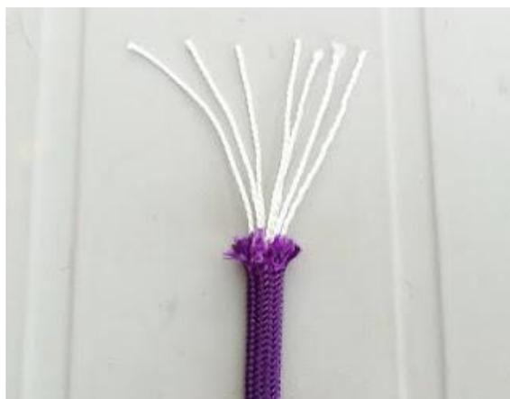
The inner strands of the core can also be removed when finer string is needed. Uses include sewing thread to repair gear, fishing line, tripwire, nets, traps, and other emergency and/or survival situations.
